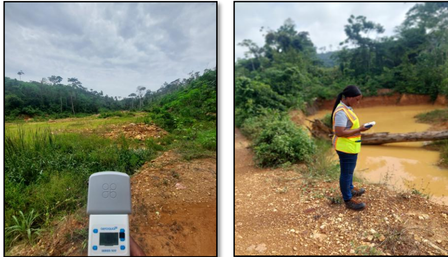
Plate 3: Monitoring with Aeroqual Series 500 (AS-500) with PM 10 and PM 2.5 Sensor head
