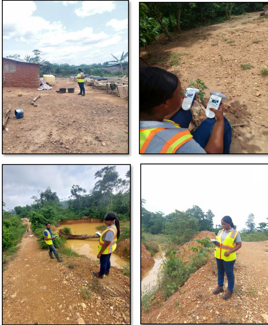
Plate 4: Aeroqual Series 500 (AS-500) with NO 2 and SO 2 Sensor head being used for monitoring
