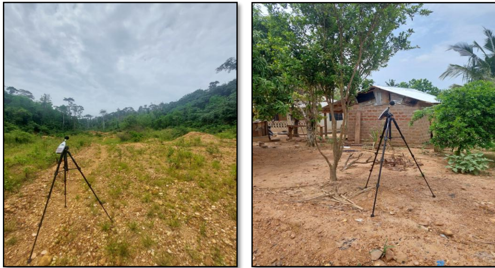
Plate 4: TSI Quest Sound Level Meter mounted for noise assessment
